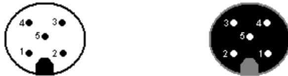
Fig. 3: Pin code: Connection plug / socket for 5-pin version
