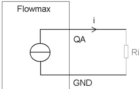
Fig. 9: The current output is active
