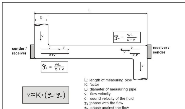
Fig. 1: Presentation of the principle of ultrasonic flow measuring
