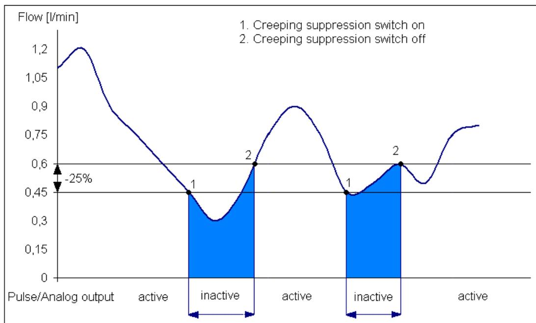
Fig. 6: Function of creeping suppression illustrated with 0.6 l/min
