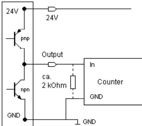
Fig. 14: Connecting Digital Output to counter
