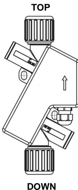
Fig. 2: Installation position of Flowmax 400i
