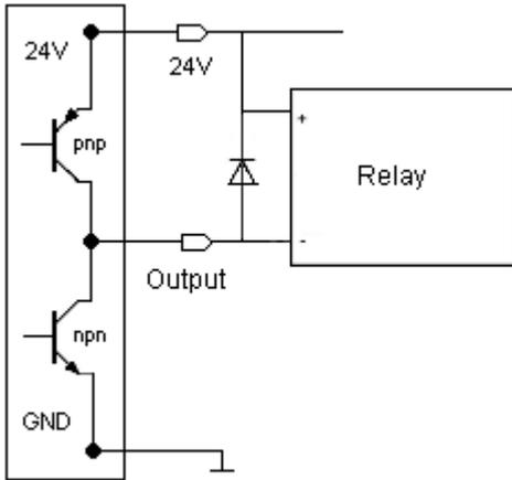
Fig. 13: Connecting Digital Output to relay
