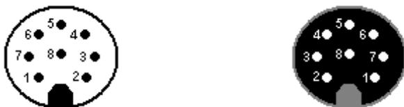
Fig. 4: Pin code: Connection plug / socket for 8-pin version
