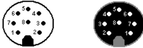
Fig. 5: Pin code: Connection plug / socket for 8-pin version
